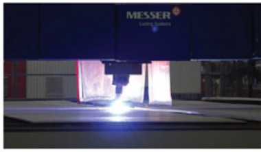
Erismet recently installed a new plasma table to support our heavy wall expansion with superior cutting edge preparation and beveling capabilities.
